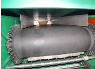
Optional segmented, spring loaded belt scraper
